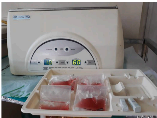
Fig. 1. Ultrasonic device and HAs placed in phloxine B solution.
