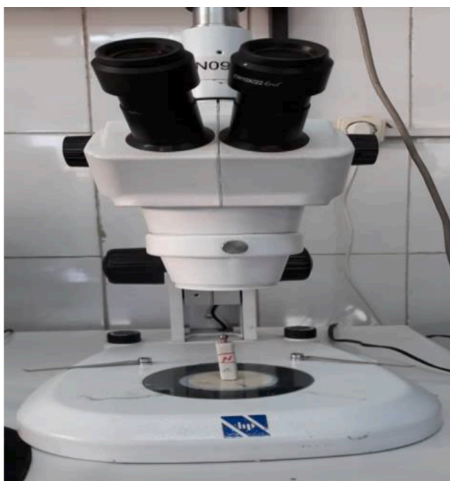
Fig. 2. Stereomicroscope and a rectangular putty mold.
