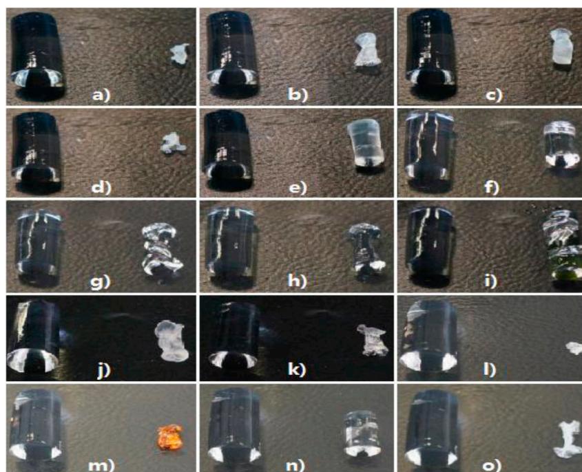
Figure 1. Pictures of shrunken gels compared to an original hydrogel. The hydrogels are placed on the left in each picture, and on the right are the gels once soaked in (a) methyl ethyl ketone (MEK); (b) isopropanol (IPA); (c) acetone; (d) 1-butanol; (e) methanol (MeOH); (f) dimethyl sulfoxide (DMSO); (g) glycerol; (h) propylene glycol; (i) ethylene glycol; (j) ethanol; (k) 1,4-dioxane; (l) propylene carbonate; (m) furfuryl alcohol; (n) N,N -dimethylformamide (DMF) and (o) acetonitrile.
