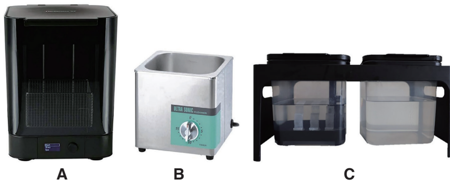
Fig. 4. Three types of devices were used for each rinsing method; (A) automated method, (B) ultrasonic method, and (C) hand-washing method.
