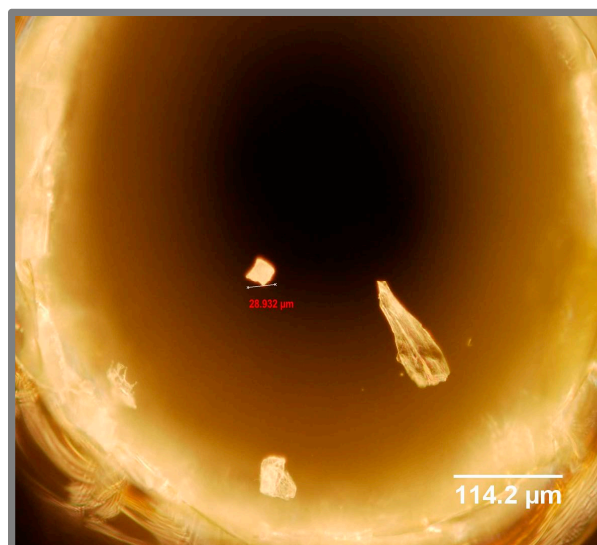
Figure 4. Microscope picture of the inlet hole made from a drilling machine with resulting shards falling off the fused silica surface.
