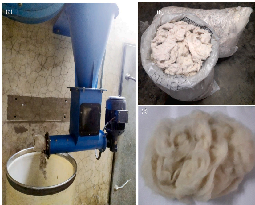
Fig. 3. (a) Rotary drum filter of ring frame section of spinning mill to collect cotton filter waste of humidification plant, (b) collected filter waste, and (c) cleaned filter waste after cleaning by Shirley analyzer.
