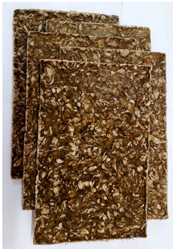
Fig. 5. Images of biocomposites produced with cotton filter waste and corn starch.
