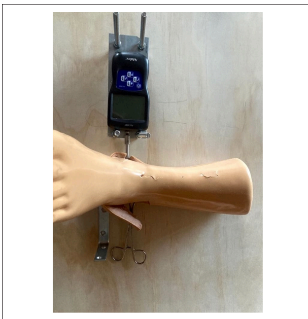
Figure 1. Biomechanical model. An industrial force gauge was fashioned to a sawbones model for simulation.
