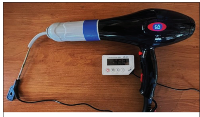
Figure 1: Checking the output temperature of the modified hair dryer with a thermometer
