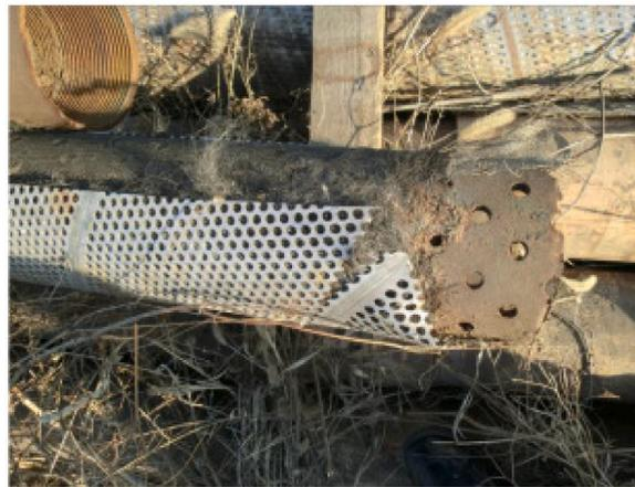
Fig. 4. Failure of metal mesh screen (MM S) [64].
