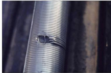
Fig. 3. Erosion of sand screen Matanovic et al., 2012.
