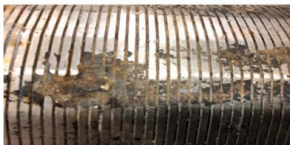
Fig. 5. Partial plugging of the wire wrap with a patchy scale layer over the screen [67].
