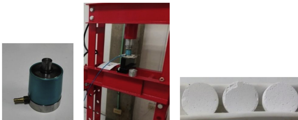
Fig. 3. Mold and uniaxial press used to obtain the green body.
