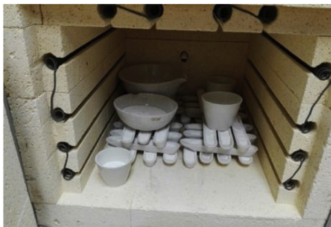
Fig. 2. TiO 2 powder samples sintered at 900 °C.
