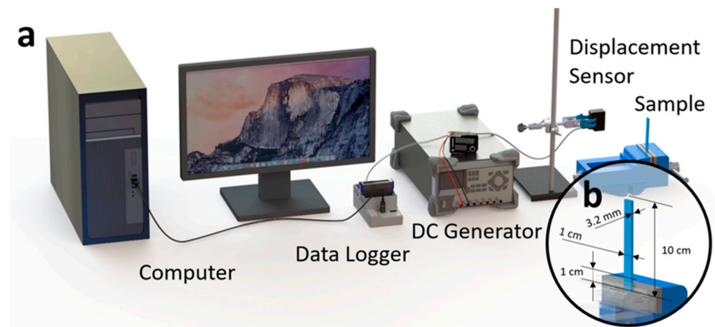
Figure 4. Apparatus used for experimental model analysis of 3D printed specimens: (a) an illustrative figure showing the connection and configuration of the experiment setup and (b) the design and configuration of the 3D printed cantilever and its clamping conditions.
