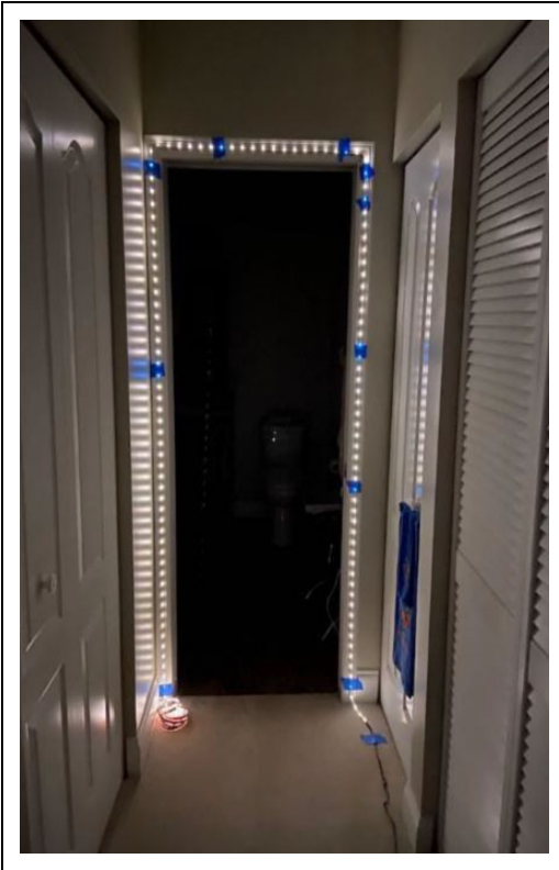
Figure 1. The LED strip lighting system was attached to the bathroom door at each participant's home.
