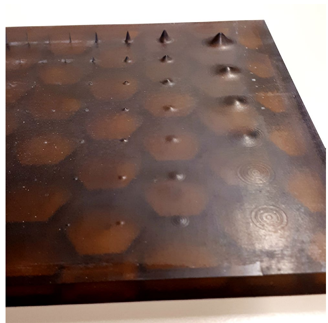
FIGURE 6 Photography of the 3D printed lesion phantom to quantify the errors induced by using the optical scanner and the analysis tool. The lesion phantom contains Gaussian-shaped lesions ranging from 0.1 to 5 mm in elevation and 0.5 to 16 mm in diameter [Colour figure can be viewed at wileyonlinelibrary.com ]
