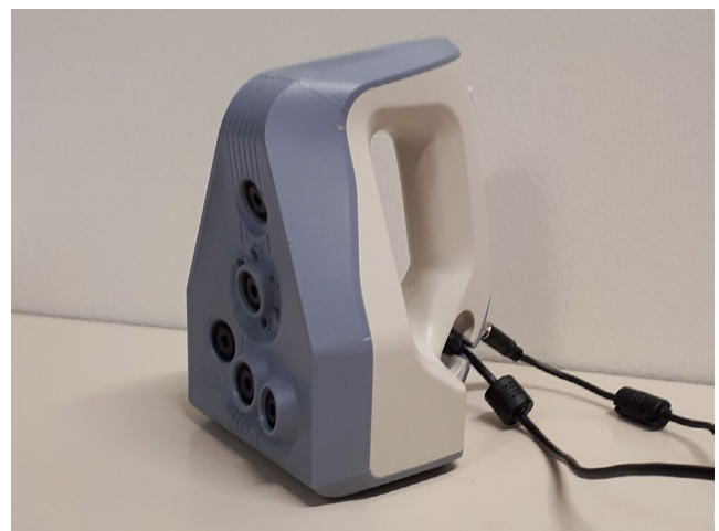
FIGURE 1 Handheld optical 3D scanner: Artec Spider, Artec 3D, Luxembourg [Colour figure can be viewed at wileyonlinelibrary.com ]
