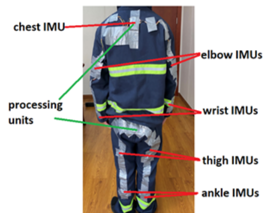
Figure 3. Placement of motion sensors that are mapped to the body parts where the motion data are critical for fall-detection computation.
