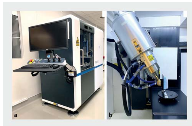
► Fig. 1 a Micro-CT scanner (Nikon Metrology NV, Leuven, Belgium). b Micro-CT scanning for whole-mount FFPE tissue block. CT, computed tomography; FFPE, formalin-fixed paraffin-embedded.
