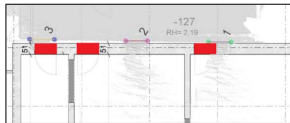
Figure 19. Comparison of the results obtained using opening detection and the ground plan (detail in Figure 17a, red: opening location in the ground plan).
