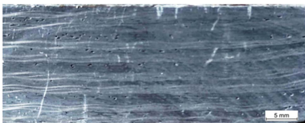
Fig. 8 Optical micrograph of the cross-section of the frontally cured CFRC plate obtained at a magnification of \times 0.65 on a Zeiss optical microscope.
