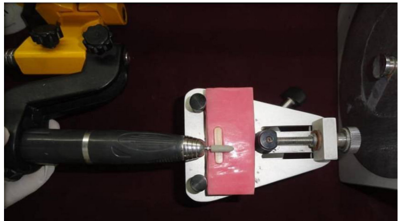
Figure 2. Polishing of a sample using the Shofu finishing and polishing system.
