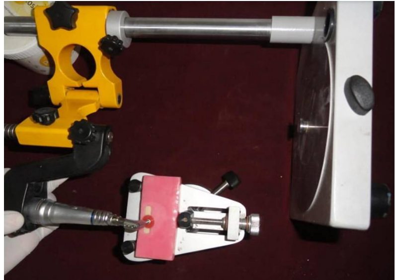
Figure 1. Polishing of a sample using Sof-Lex discs.
