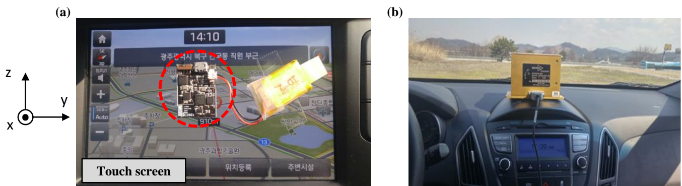
Figure 3. Measuring setup of driving vibration on the touch screen in vehicles. (a) E2BOX's EBIMU24GV3. (b) Crossbow's VG700CB-200.
