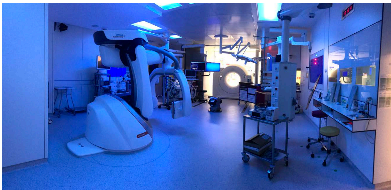
FIGURE 5. Photograph of a hybrid operating room. In this case, computed tomography, magnetic resonance imaging, and cone-beam computed tomography systems (Siemens Healthineers, Forchheim, Germany) are combined in the same suite.
