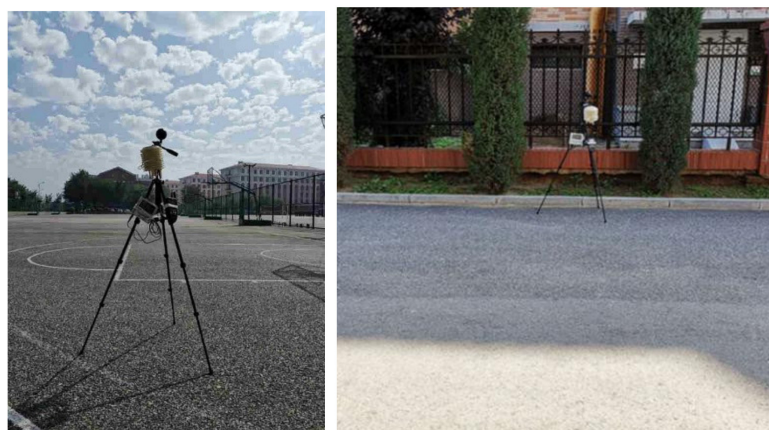
Figure 3. Measurement of thermal environment parameters under the sun (left) and under shade (right).
