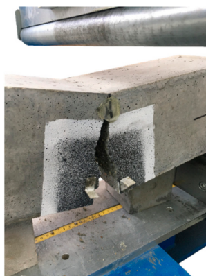
Figure 13. PC_1 beam without fibers after the three-point bending test.
