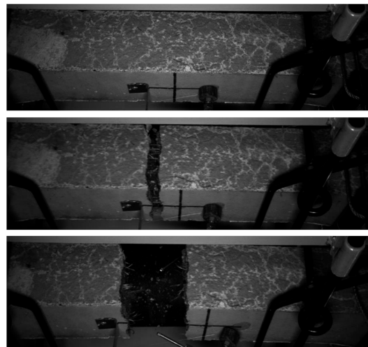
Figure 19. Cracking of PM_2 dog-bone specimen during the tensile test.
