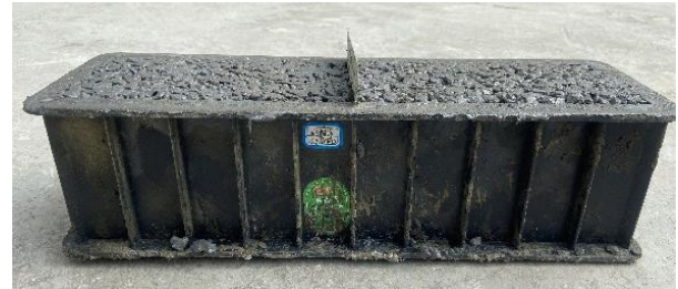
(b) Prepared fracture toughness test specimen
