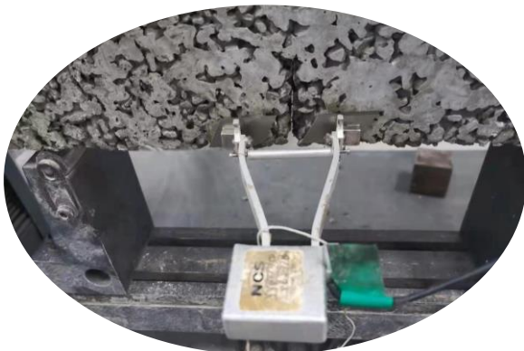
(c) Double-cantilever clip-in displacement gauge contacts
