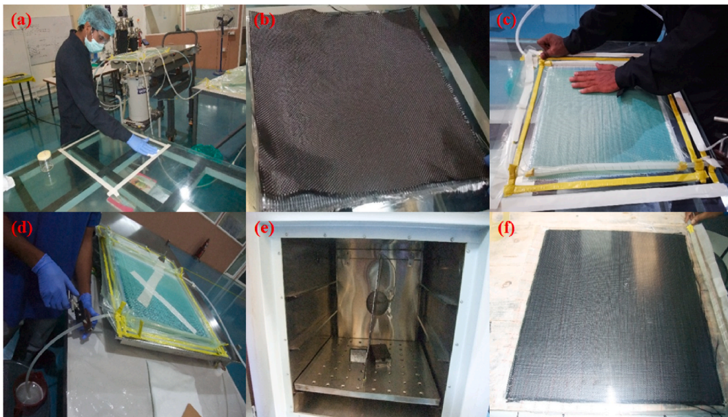
Fig. 1. Fabrication of composite laminate: (a) mold preparation, (b) fiber stacking, (c) vacuum bagging, (d) connecting tubes for matrix flow, (e) post curing, and (f) composite laminate.
