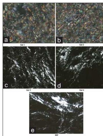
**Figure 2:** Pictures from the optical microscope at  $\times 500$  magnification with polarized light of the ciprofloxacin (1 and 2), gentamicin (3 and 4) and REF monoolein water gels
