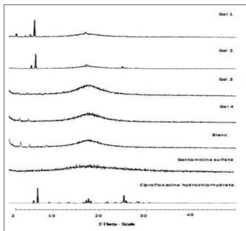
**Figure 3:** X-ray diffraction spectra of ciprofloxacin hydrochloride and gentamicin sulfate powders, ciprofloxacin (1 and 2), gentamicin (3 and 4) and REF (Blanc) monoolein water gels
