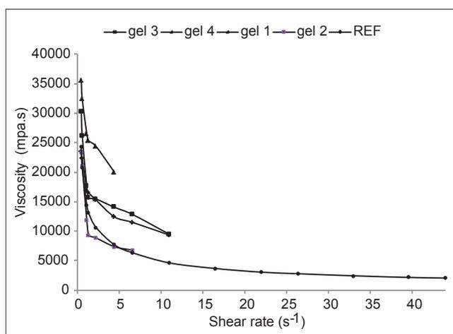
**Figure 5:** Rheograms of the ciprofloxacin (1 and 2), gentamicin (3 and 4) and REF monoolein water gels, measured at 37 °C with a SC4-25 spindle ( $m \pm SD, n = 3$ )
