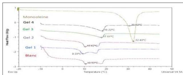
**Figure 4:** Differential scanning calorimetry heating curves for glycerol monooleate (monooleine), ciprofloxacin (1 and 2), gentamicin (3 and 4) and REF (Blanc) monoolein water gels recorded during the first heating.
