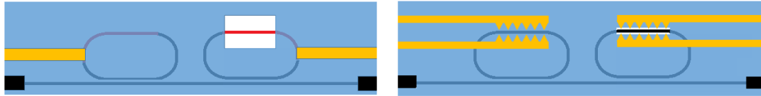
Figure 7. Ring resonator layout. Each sensor consists of two ring resonators (dark blue) coupled to a common bus waveguide (dark blue) using directional couplers. One ring is completely covered with \text{SiO}_2 (light blue) and acts as a reference to control for ambient temperature. The two variants differ in terms of using doped waveguides (left) and coplanar electrodes (right) for dielectrophoresis.
