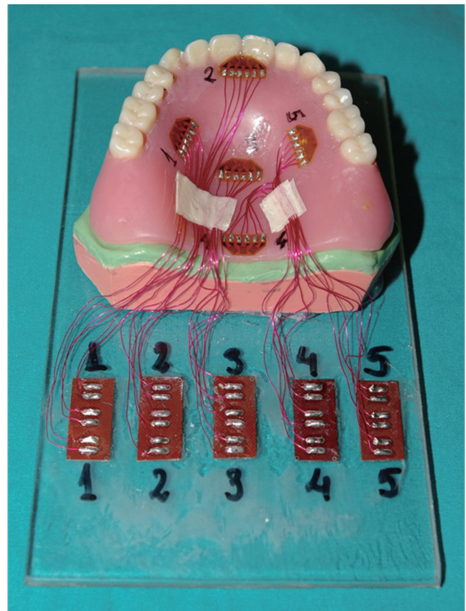
Fig. 1. Positions of the strain gauges on a maxillary complete denture.
