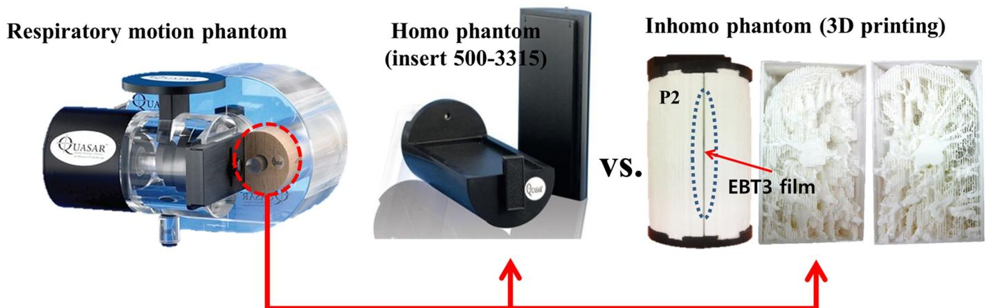
**Fig 2. 4D phantom with 3D printed lung phantom.** The inserts are either a 3D printed lung phantom (inhomogeneous) or a homogeneous phantom.
