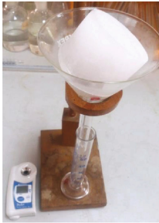
FIGURE 3: Partial melting of formed ice fraction of PFC; melted volume collected in 10 mL fractions.
