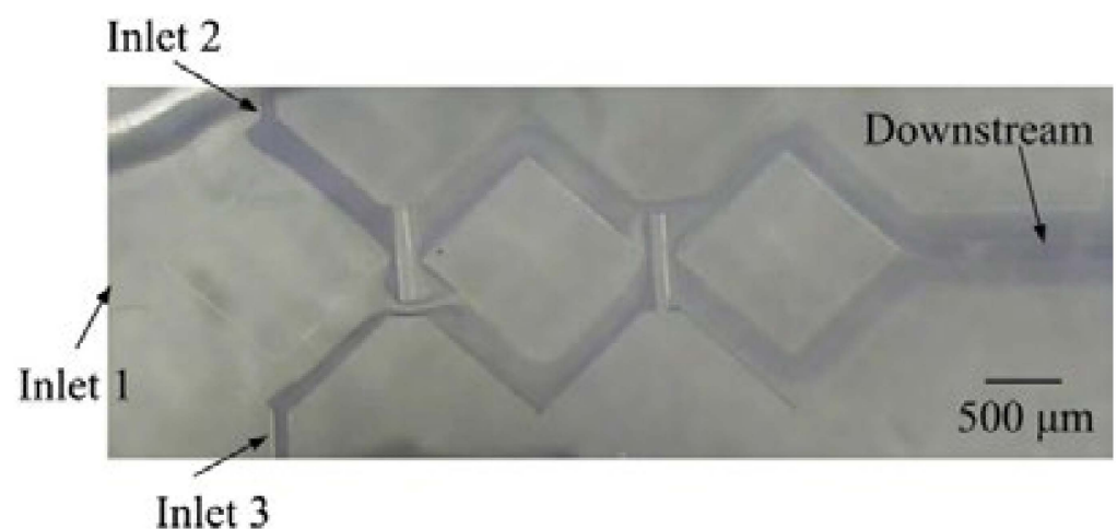
Figure 22. Optical micrographs of fluid mixing in the rhombic micromixer with a gap ratio of 1/8 at Re = 20 . The top view image is recorded by a Charge-coupled Device (CCD) camera.
