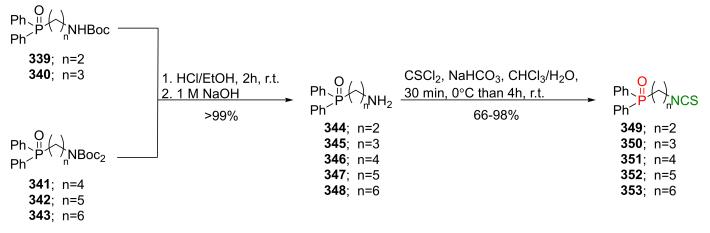
Figure 40. Synthesis of (*w*-isothiocyanatoalkyl)diphenylphosphine oxides 349–353.
