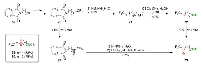
Figure 20. Synthesis of trifluoromethyl (73) and trifluoroethyl (75–76) analogs of SFN.
