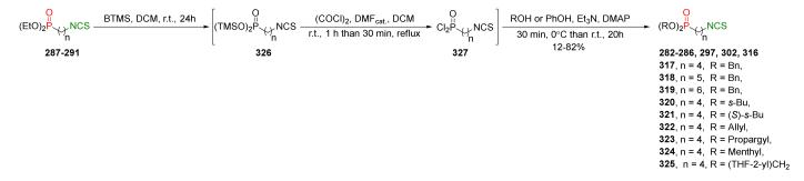
**Figure 38.** Conversion of diethyl  $\omega$ -(isothiocyanato)alkylphosphonates **287–291** into dialkyl or diphenyl  $\omega$ -(isothiocyanato)alkylphosphonates **282–286**, **297**, **302**, **316–325**.
