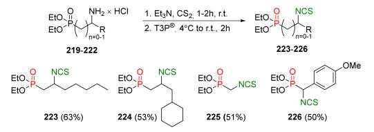
Figure 35. Synthesis of  $\alpha$ - and  $\beta$ -dialkoxyphosphoryl isothiocyanates 223–226.
