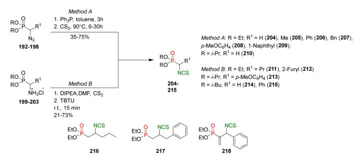
Figure 34. Synthesis of  $\alpha$ - and  $\beta$ -dialkoxyphosphoryl isothiocyanates 204–218.
