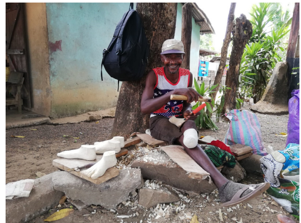
Fig. 7. The prosthetic foot is made from wood, in the size of the person's foot, produced by a local hospital patient who is specialized in wood carving.
