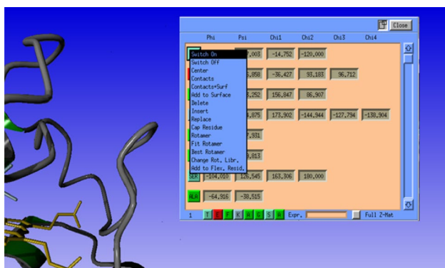
Fig. 7 The Z-matrix editor pop-up window. Each residue is represented by a column with a button labelled with its three letter amino acid code and entry fields for the \phi , \psi , \omega angles. Clicking the button brings up a pop up menu containing residue manipulating options
