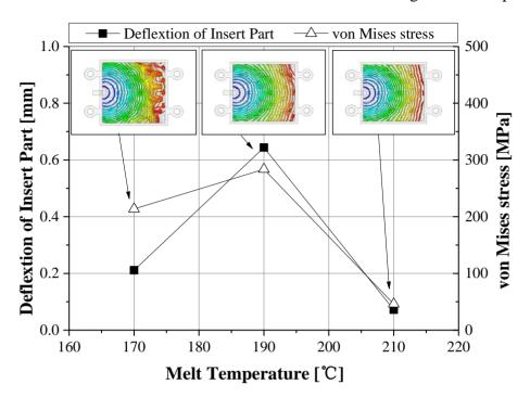
Figure 10. Deformation of insert and von Mises stress according to melt temperature.
