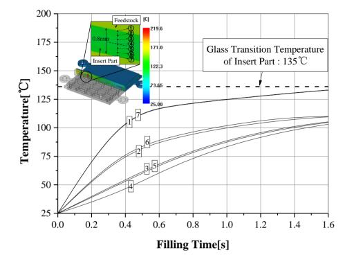
**Figure 14.** Distribution of the cross-section temperature in the sacrificed polymer insert for 17-4PH feedstocks.
