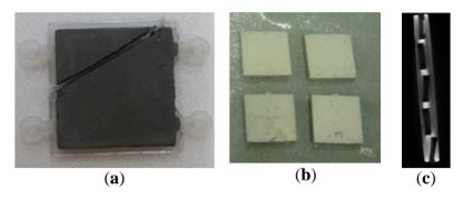
Figure 16. SEM images for the part at each phase. (a) green part; (b) brown part; and (c) sintered part.
