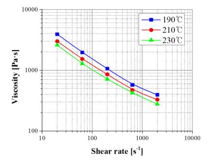
Figure 2. Result of the measured viscosity of 316 L feedstocks.
