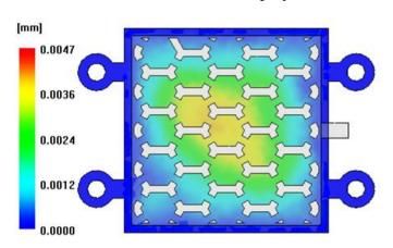
Figure 13. Distribution of deformation in the sacrificed polymer insert for 17-4PH feedstocks.
