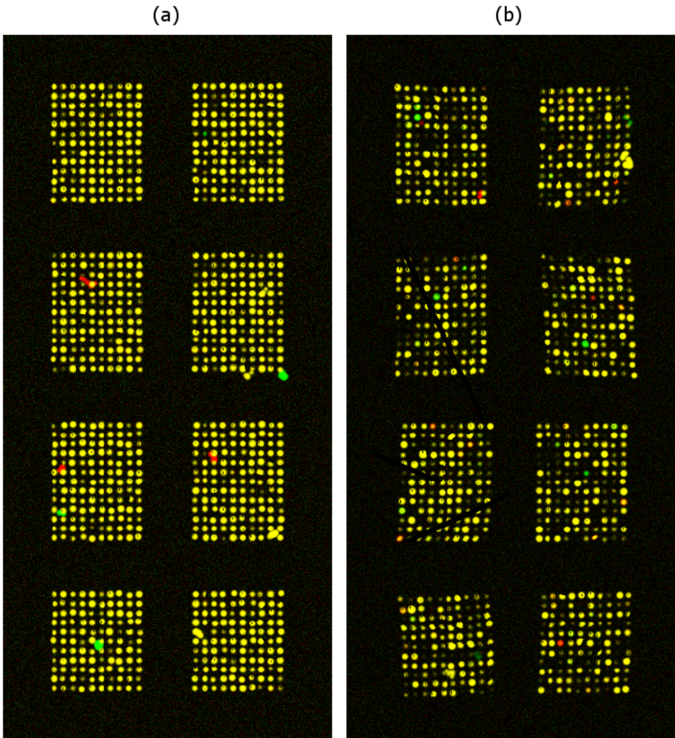
Figure 8 Simulated spotted microarray slide images. Simulated slide images at time instants (a) 10 and (b) 200 minutes. Several error sources, like spot size and shape variation and bleeding are included in simulation. On the slide image on the right (b) also unideal subarray alignment and scratches are introduced.
