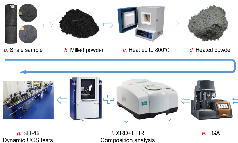
Figure 1. (a–g) Schematic workflow for sample preparation and analysis.
