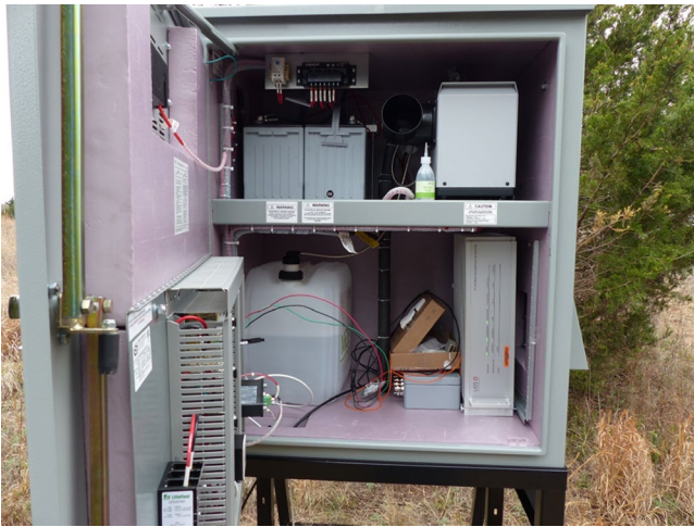
FIGURE A2 A photograph of the weatherproof housing and fueling system (upper shelf and lower left shelf) that supported our distributed temperature sensing system's controller (lower right shelf) approximately 15 km west of Stillwater, Oklahoma, USA
