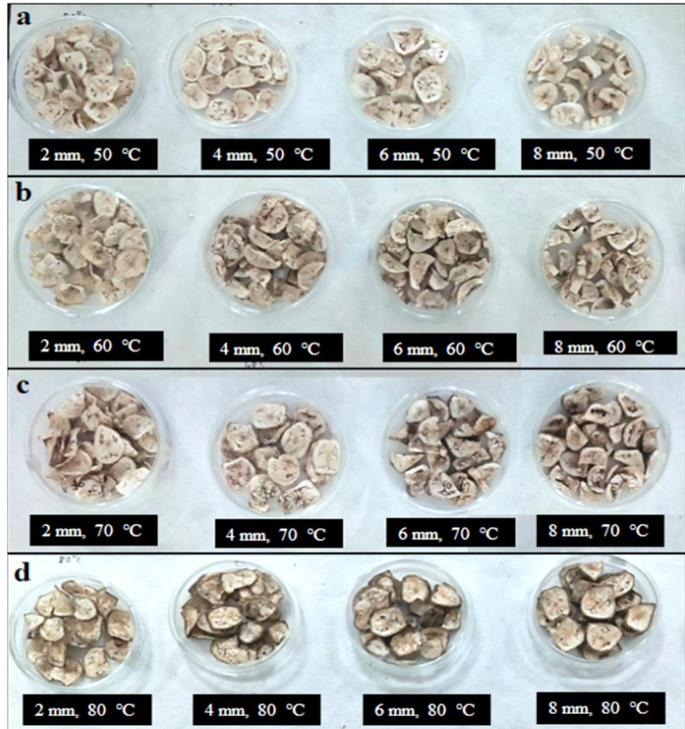
**Figure 1.** Convective hot-air-dried plantain banana slices with thicknesses of 2, 4, 6, and 8 mm dried at 50 °C (a), 60 °C (b), 70 °C (c) and 80 °C (d).
