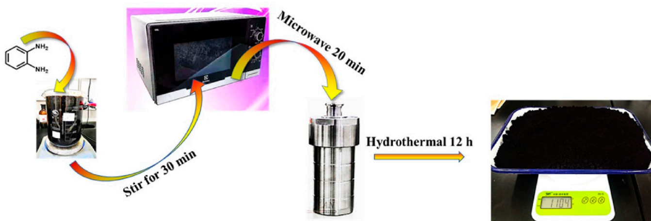
Figure 1. The synthesis process of C-dots 606 from o -PDA at a kilogram scale (1.104 kg) with high yield by a combined microwave-hydrothermal process (reprinted with permission from [50], 2022, Elsevier).
