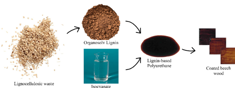
Scheme 1. Overview of the general procedure for the preparation of the Organosolv lignin-based PU coating.
