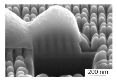
**Figure 5.** The SEM image of the interface between bacteria and the 100 *O* nanopattern. The depth of direct penetration of the nanopillars into the bacterial cell wall (about 100 nm) far exceeds the average cell wall thickness of *S. aureus* (i.e., 10–20 nm).
