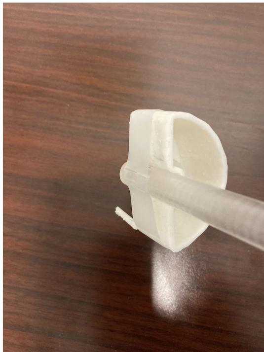
**FIG. 2.** 3D-printed cement container attached to micro-chamber phantom insert.
