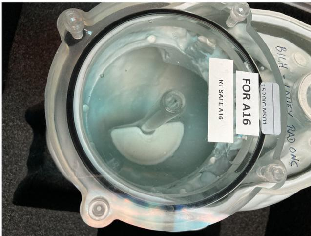
**Fig. 4.** Kyphoplasty cement in anthropomorphic phantom adjacent to ion chamber insert.
