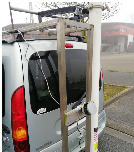
Figure 11. VLP-16 LiDAR mounted on a vehicle toward the ground.
