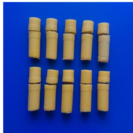
Figure 4. The implant–abutment assemblies placed in putty to the interface in order to minimize the incident of bonding of radiotracer to their external surfaces.
