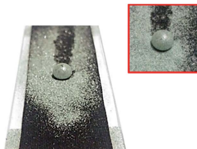
Fig. 10 Photos of the polypyrrole deposited and hydrophobic coated cotton fabric after scattering silicon carbide particles on the surface and cleaning with water droplet.
