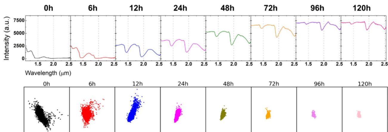
**Fig. 3.** Spectrum of drying cement (top) and plot of dimensionality-reduced data achieved via linear discriminant analysis (LDA) (bottom).
