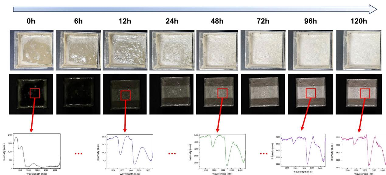
**Fig. 2.** Visible (top) and near infrared images (middle) captured using spectral camera. Spectrum (bottom) at a certain time was obtained at central point of image.
