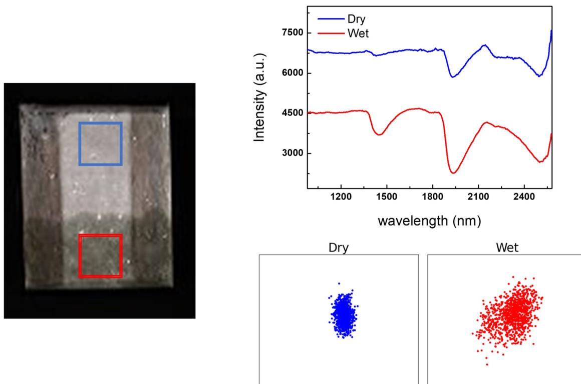
**Fig. 5.** (Left) NIR image of sample with different moisture contents at top and bottom. (Right-top) Spectra obtained from measured image. (Right-bottom) Data dimensionally reduced via LDA. Data obtained from wet region (red), which deviate slightly from those obtained from dry region (blue).
