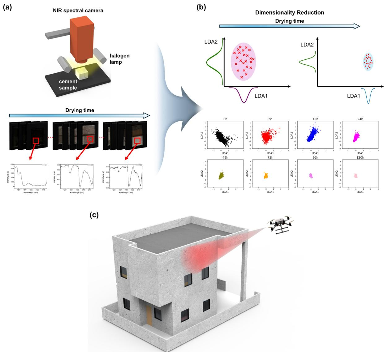
**Fig. 1.** (a) Schematic illustration of spectral imaging for dryness of cement-based mixture. (b) Schematic illustration of dimensionality reduction processes on spectral images (top) and graphs of dimension-reduction analysis representing as a drying time goes (bottom) (c) Schematic of real-time monitoring on the status or dryness of cement-based building using a drone with a hyperspectral imaging apparatus.
