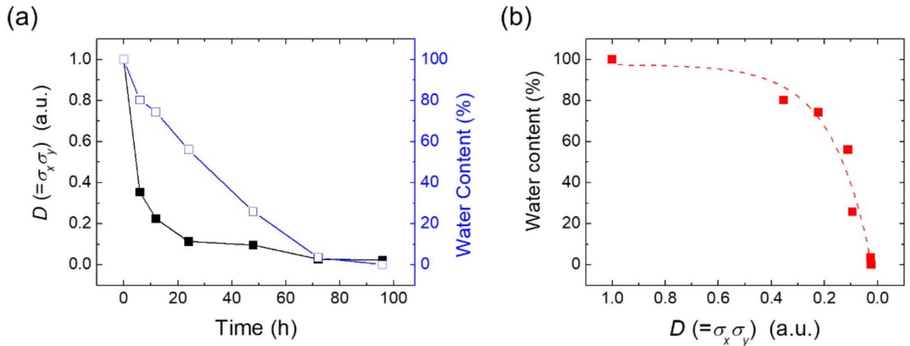
**Fig. 4.** (a) Plot of  $D$  parameter (product of  $x$ - and  $y$ -standard deviations) and water content in cement-water mixture sample as a function of drying time. (b) Plot of water content in cement-water mixture sample  $t$  as a function of  $D$  parameter.
