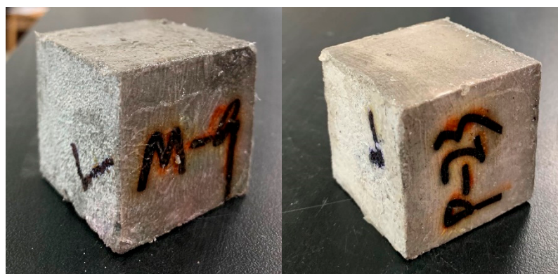
Figure 1. Sealed specimens in the experimental work, the “ \checkmark ” marked surface was the only unsealed surface.
