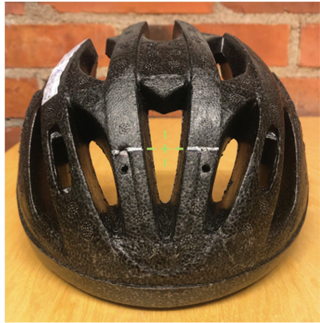
Figure 7. Center of impact projection and testing sites on a helmet test specimen.
