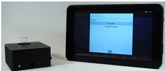
Fig. 3. NECi open-source portable photometer with tablet PC running the NECi phosphate soil analysis app. The photometer is shown with a 1.5 mL disposable cuvette installed, which is 1 cm in path length, which provides a measure of dimensions of the photometer (8 × 7.2 × 3.5 cm). The NECi photometer is connected to the table PC by bluetooth prior to taking readings. The setting menu allows the user to blank the photometer prior to taking readings.
