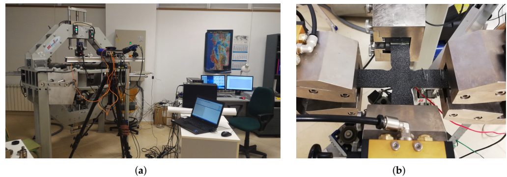
Figure 1. Triaxial testing facility at University of Castilla-La Mancha (UCLM, Spain): (a) triaxial testing machine. (b) CFRP cruciform specimen being tested under biaxial tensile–tensile loading.
