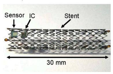
**Figure 5.** An example of a remote-powered blood pressure sensor. Power is received via the stent, which doubles as an antenna, to power the sensor and processing integrated circuit (IC). Reprinted with permission from Reference [110].
