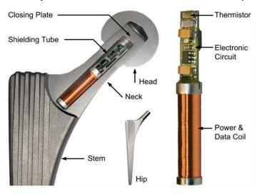
**Figure 4.** A smart hip implant featuring a telemetered temperature sensor to detect loosening. CC BY [85].
