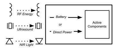
**Figure 3.** Methods of remote power for implantable devices. RF energy (top-left) can be transmitted through inductors; ultrasound energy (middle-left) can be transmitted through piezoelectric materials; near-infrared (NIR) light (bottom-left) can be transmitted via light-emitting diodes (LEDs) and photoreceptors. The received energy may be either stored in a battery or used directly.
