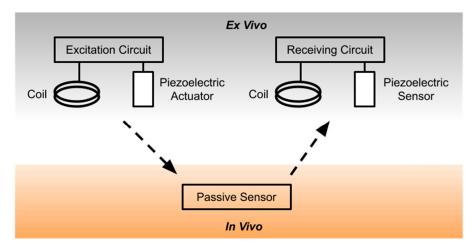
**Figure 2.** The design of a generic passive interrogator. A signal is generated in the excitation circuit and transmitted at radiofrequency (RF) using an inductive coil or at ultrasound frequencies using a piezoelectric element. The reflected signal is received by a receiving circuit using a matching coil or piezoelectric element.
